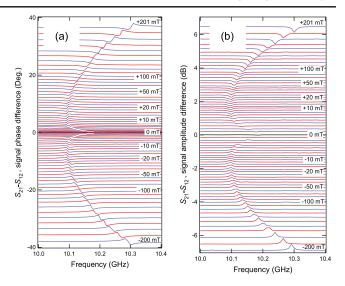
FIG. 3 (color online). Differences in (a) phases and (b) amplitudes between  $S_{21}$  and  $S_{12}$  around 10 GHz of the MCh metamolecule under dc magnetic fields from 0 mT to  $\pm 200$  mT.
