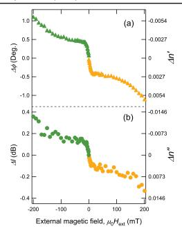
FIG. 4 (color online). Differences in (a) phases and (b) amplitudes are plotted as a function of  $\mu_0 H_{\rm ext}$ . Evaluated differences in the index of refraction are also indicated from the right axes.
