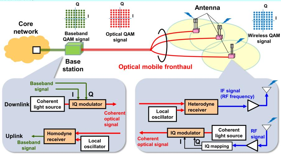
Direct conversion between optical and microwave frequencies while maintaining coherence
