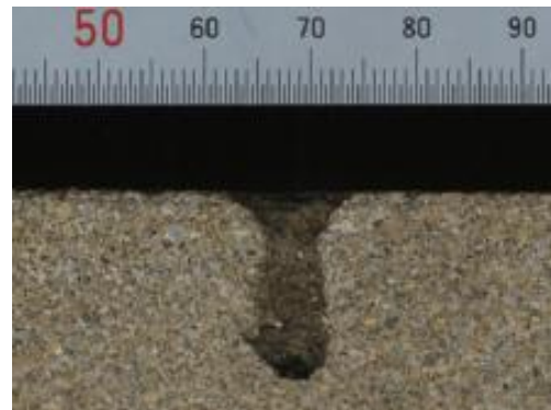
Fig. 2 Cross-section of view of borehole.
