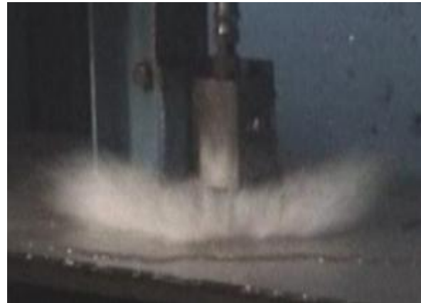
Fig. 3 Experimental result of jetting to a steel plate.
