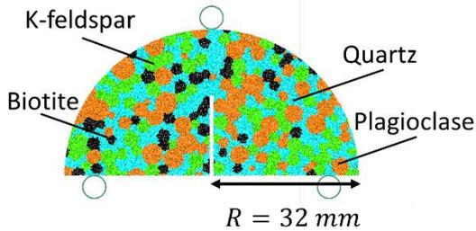
**Fig.7 An example of numerical SCB model with radius 32mm**
