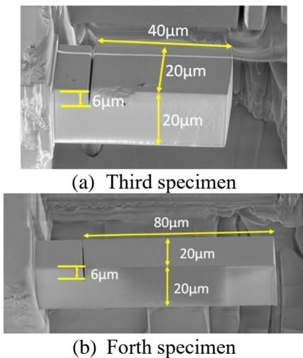
**Fig.5 SEM images of different dimension specimens; (a)third specimen, (b) forth specimen.**
