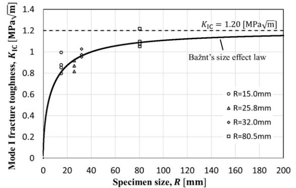
Fig.2 Mode I fracture toughness of Inada granite with various size
