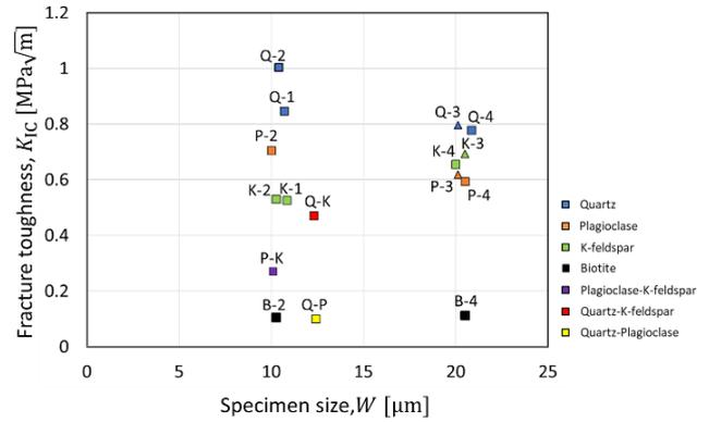
**Fig.6 All the results of MFT tests, and relation between  $K_{IC}$  and specimen size**
