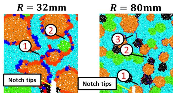
**Fig.9 Bonding state just after peak load**
