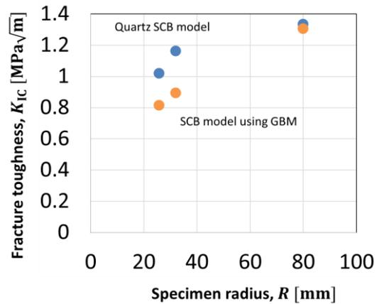
**Fig.8 Comparison between quartz SCB model and GBM SCB model.**
