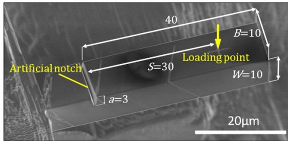
**Fig.4 SEM images of MFT specimen with standard dimensions.**
