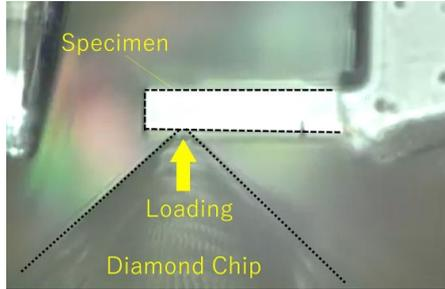
**Fig.3 Loading state of MFT test.**
