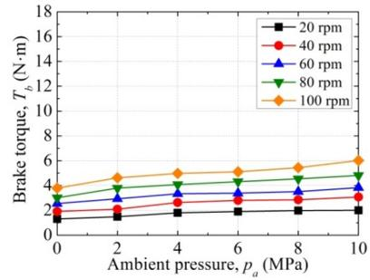
Fig. 8 Relation between the ambient pressure and the brake torque of the nozzle system for five rotational speeds of the nozzle system ( $s = 12.0 \text{ mm}^2$ ,  $T = 50 \text{ }^\circ\text{C}$ ).
