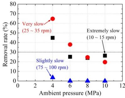
Fig. 7 Relation between the ambient pressure and the removal rate for three rotational speeds of the nozzle system.
