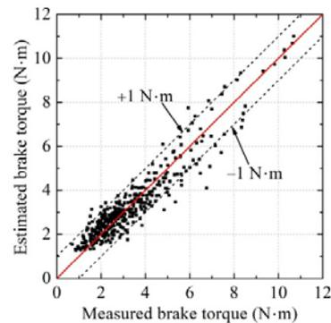
Fig. 10 Comparison between the measured and the estimated brake torque of the nozzle system.
