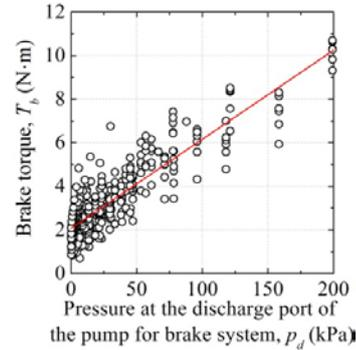
Fig. 9 Relation between the pressure at the discharge port of the pump for brake system and the brake torque of the nozzle system.
