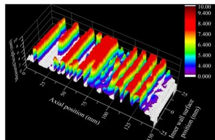
Fig. 6 Scanned surface images of the specimens after the scale removal ( $p_a = 4, 10$  MPa,  $\omega = 10 \sim 15$  rpm).
