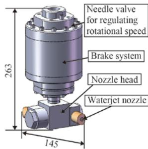
Fig. 2 Low-speed self-rotating nozzle system.
