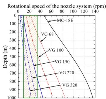
Fig. 11 Relation between the depth and the rotational speed of the nozzle system for six kinds of oil ( $s = 12.0 \text{ mm}^2$ ).
