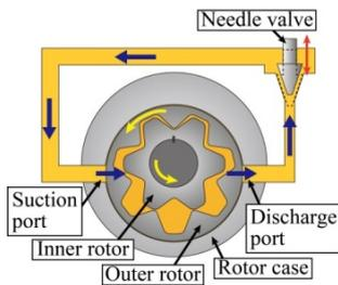
Fig. 3 Schematic illustration of the hydraulic pump and fluid path for the brake system.
