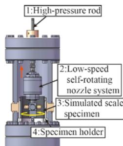
Fig. 5 Vertical cross-section of the pressure vessel in the scale-removal experiment.
