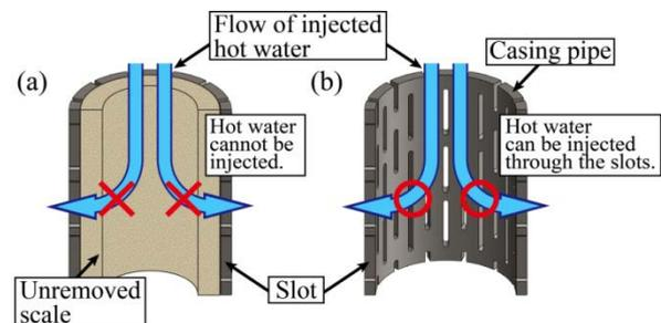
Fig. 1 Schematic illustrations of the vertical cross-section of the slotted casings ((a) before scale removal and (b) after scale removal).
