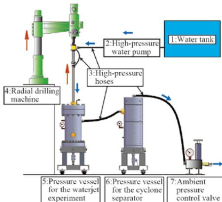
Fig. 4 Schematic illustration of the experimental system.
