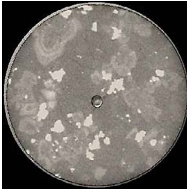
Fig. 3 X-ray CT image of specimen after experiment under ductile condition (450 °C, 30 MPa).
