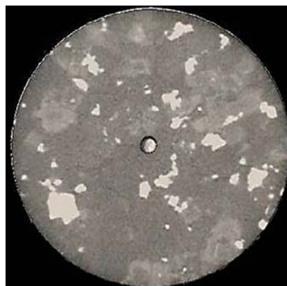
Fig. 7 X-ray CT image of specimen after experiment under ductile condition (450 °C, 40 MPa).
