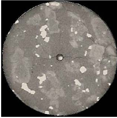
Fig. 8 X-ray CT image of specimen after experiment under brittle condition (360 °C, 40 MPa).
