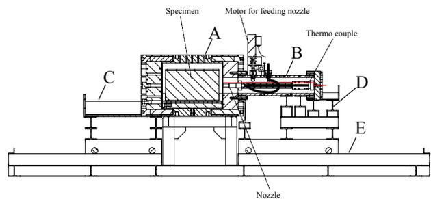
Fig. 1 Vertical cross section of experimental apparatus.
