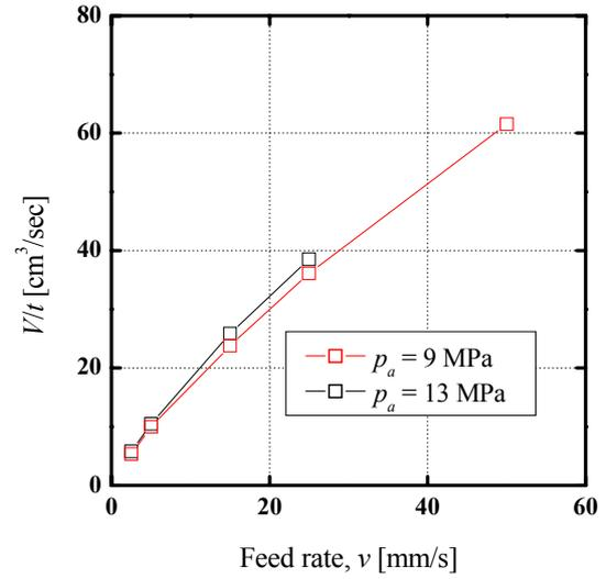
Fig. 4 Effect of feed rate  $v$  on excavation rate  $V/t$ .
