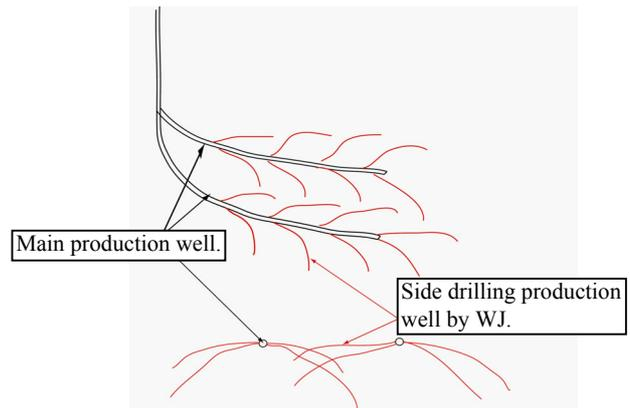
Fig. 8 An example of layout of side drilling with WJ from main production well.
