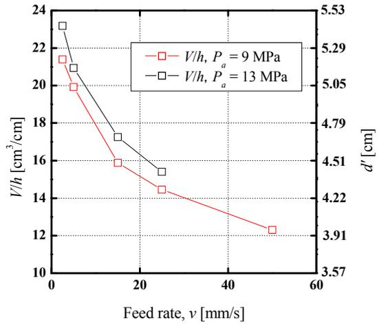
Fig. 5 Effect of feed rate  $v$  on  $V/h$  and equivalent hole diameter  $d'$ .
