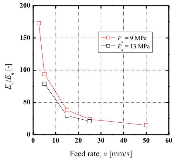
Fig. 7 Relation between feed rate  $v$  and  $E_w/E_n$ .
