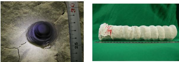
Fig. 3 An example of a borehole after drilling experiment ( $p_a = 9$  MPa,  $v = 2.5$  mm/s).
