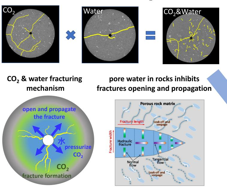
CO<sub>2</sub> & water fracturing is still effective with the pre-existing pore water and is particularly effective in porous volcanic rocks.
