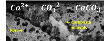
In order to utilize reservoirs in the most efficient, safe, and secure manner, we invented a method to promote CO2 geological storage and mineral fixation. [patent application2023-51335]
