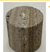
Rocks that have undergone clayey alteration and oxidative alteration Contains the clay mineral montmorillonite **Biodegradable chelating agent GLDA** dissolves minerals to improve permeability
