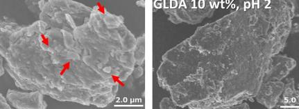
Montmorillonite dissolved in GLDA **Confirmation of pore formation**
