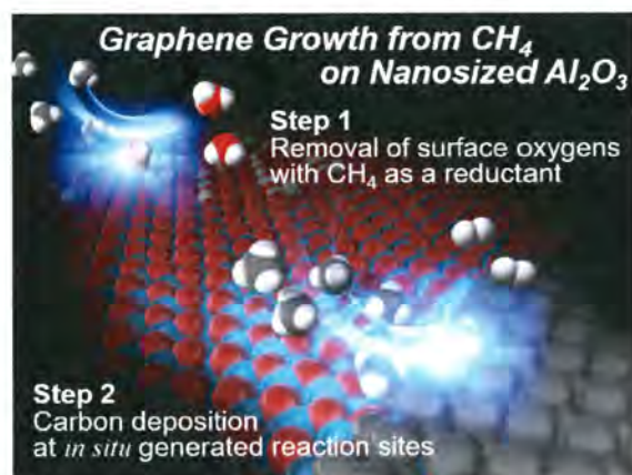
Figure 2. Schematic of the gas-phase reaction of CH 4 into single-walled carbon sheet on an ANP.
