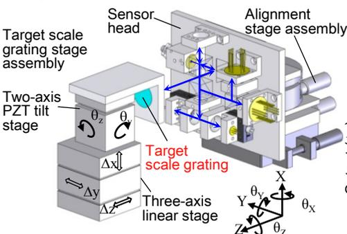
6-DOF surface encoder can provide nm and sub-arcsec resolutions for 6DOF position sensing.
