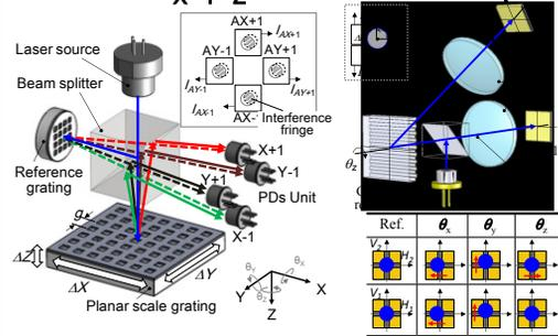
Constructed sensor head and fabricated scale grating
